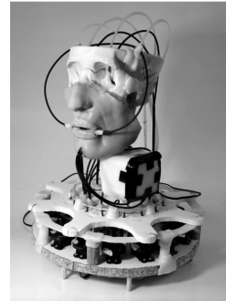
Image of Anton - Animatronic tongue and vocal tract model created by Robin Hofe, http://staffwww.dcs.shef.ac.uk/people/R.Hofe/anton/tongue.html
